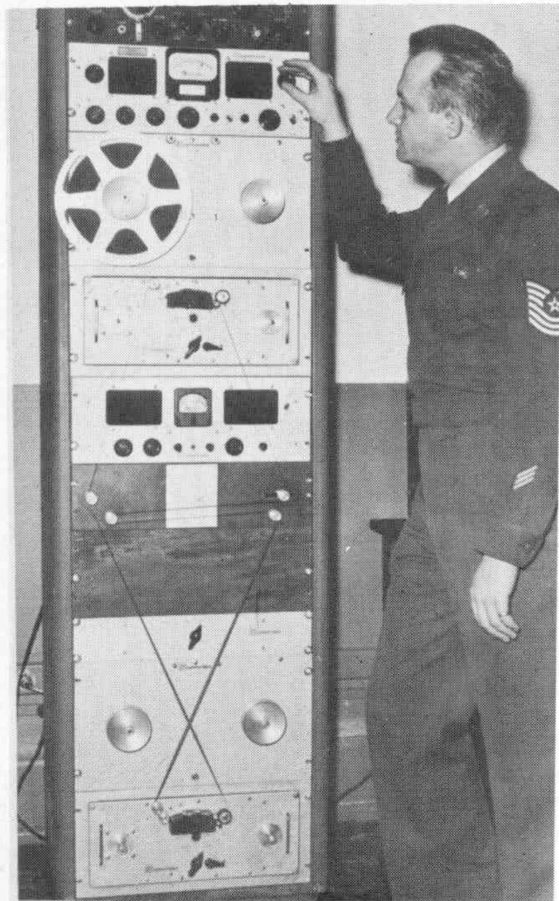
Recorder setup for the time-delay loop showing the two Magnecorders, special panel with insion roller and ampliier which form the basis of method described by Lt. Jesse C. Durham, USNR, for AFRS "Editing without Cutting Tape."
