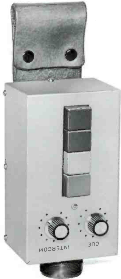
Unique "belt box" station for studio floormen. The box hangs on his trousers belt and connects him with the intercom system without restricting mobility. Four pushbuttons give him two-way communication with as many stations on the intercom system.
