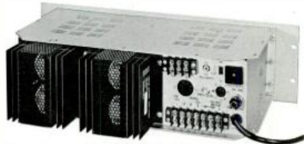
Rear view, basic amplifier. Note barrier-strip connections and power outlet. "Lo-Cut" switch at upper right, next to outlet.
