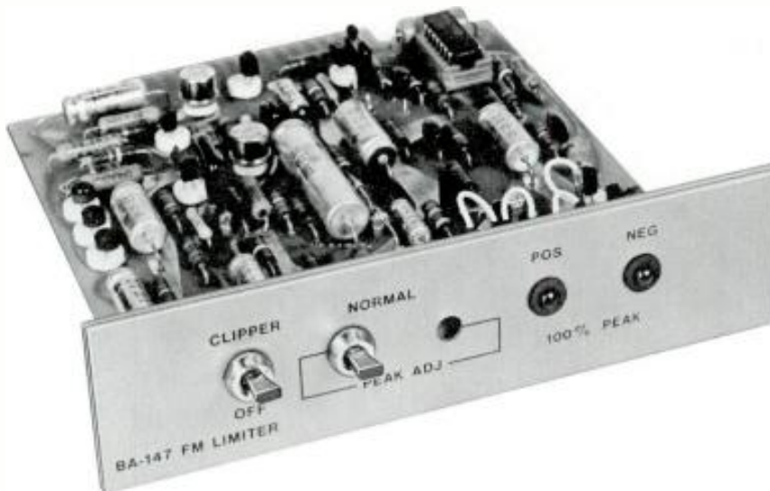
This module plugs into a BA-146 to convert it to a BA-147 Limiter/Clipper for FM, SCA and TV aural use.
