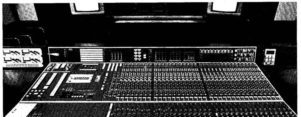
STUDER audio mixer 904 with VCAs and built-in system controller SC 4016.
