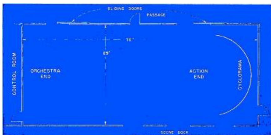
Fig. 2. Plan view, Studio A, London Television Station.
