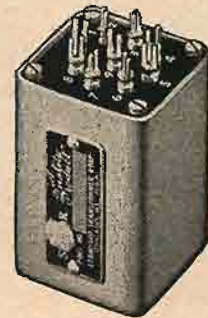
HIGH-FIDELITY INPUT TRANSFORMER, WF-20, for low impedance microphone, pickup or line to grid. Primary impedance 50, 125/150, 200, 250, 333, 500/600 ohms. Secondary impedance 50,000 ohms. Frequency response 30-20,000 cps. ± 2 db. Negligible harmonic and intermodulation distortion. Grey enamel cast case with phenolic terminal board and tapped holes for flush mounting. 2" high by 1½" square.
