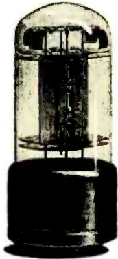
The controlling quartz crystal vibrates in vacuum at 100,000 cycles per second. The standard is powered by storage batteries, with steam turbo-generator standing by, just in case of emergency.
