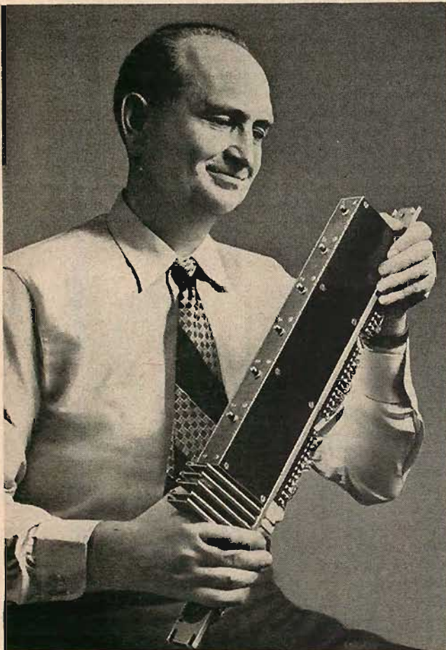
Laboratories engineer examines Transistor oscillator. It is used in Englewood, New Jersey, where 10,000 subscribers can personally dial distant cities. Transistors generate the signals which carry the dialed numbers to other towns and cities. Other uses are in prospect.
