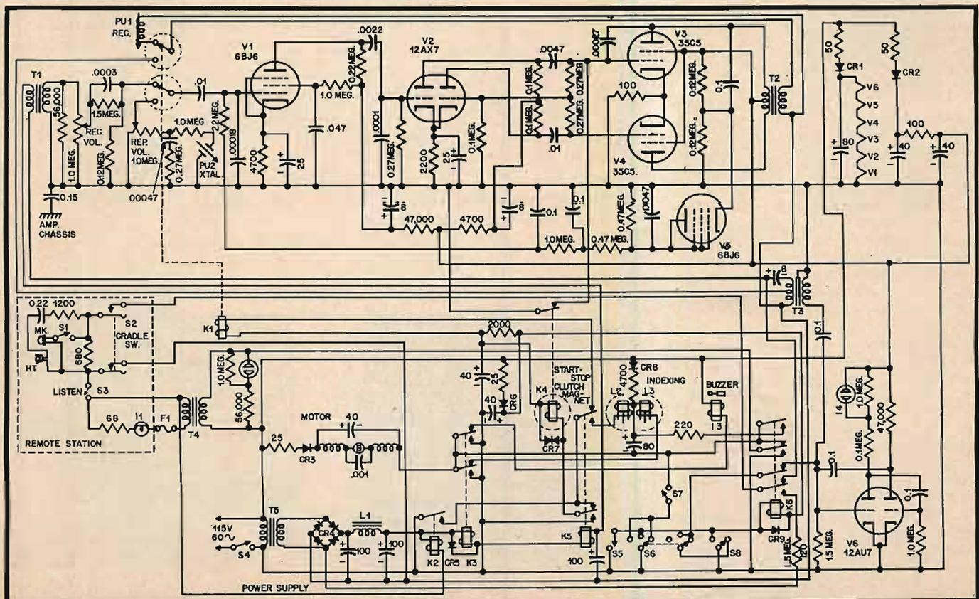
Fig. 12. Schematic of the TeleVocewriter, including amplifier, control circuits, and a remote station.
