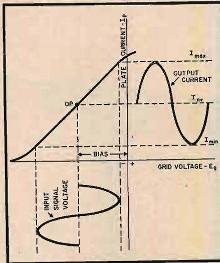
Fig. 12—21. Transfer characteristic illustrating Class  $A_1$  operation. Plate current flows during the entire cycle, and the input signal is neither allowed to engage the curved lower portion of the  $I_p - E_g$  curve, nor to drive the grid positive.
