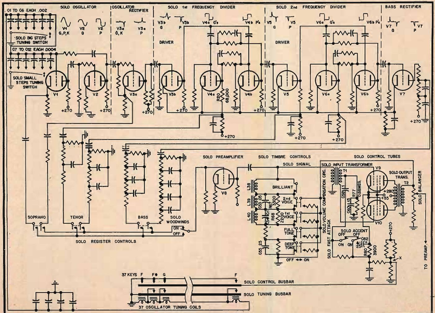
Fig. 5. Simplified schematic of the solo section showing the tone-forming circuits which follow the oscillator and the frequency-dividers.
