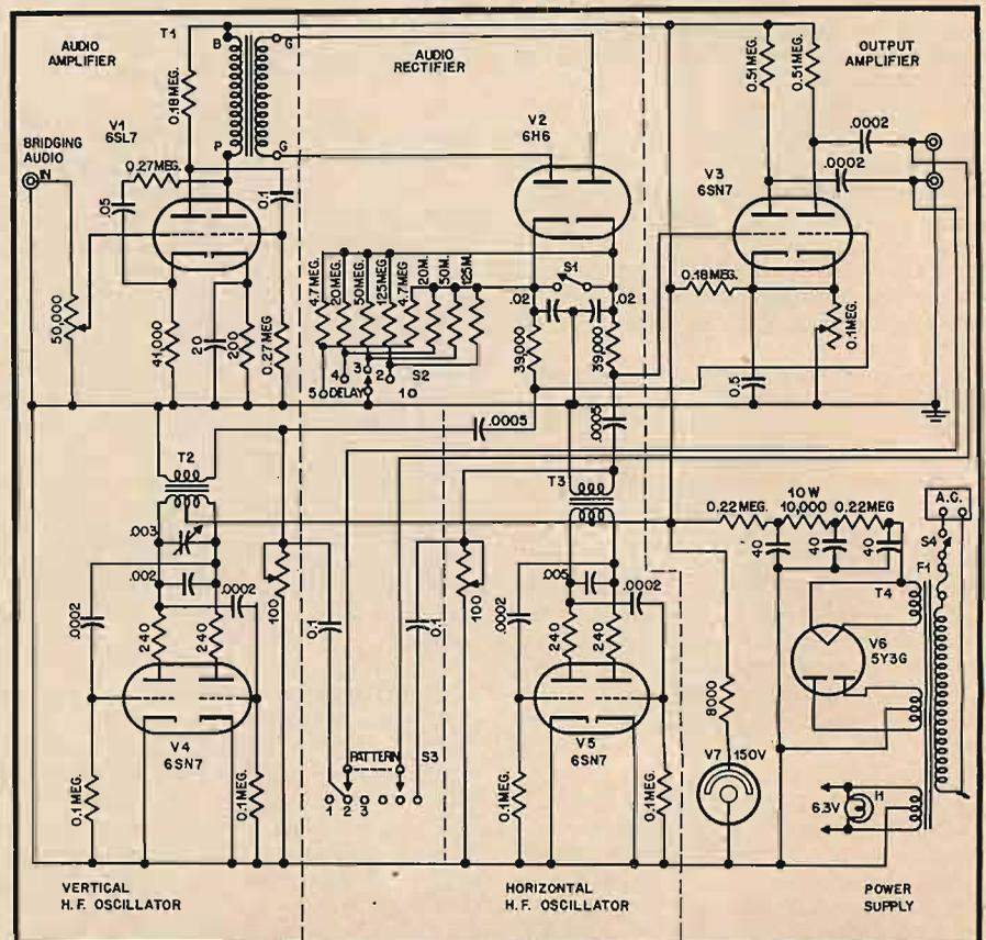
Fig. 4. Complete schematic of the cathode-ray Volume Visualizer.
