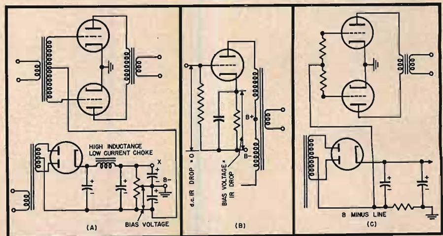
Fig. 12-23. Methods of providing grid bias voltage. (A) Fixed bias from separate power supply. The point marked X is sometimes used to supply plate voltage for low-current voltage amplifiers. (B) Cathode or self-bias. (C) Back bias.
