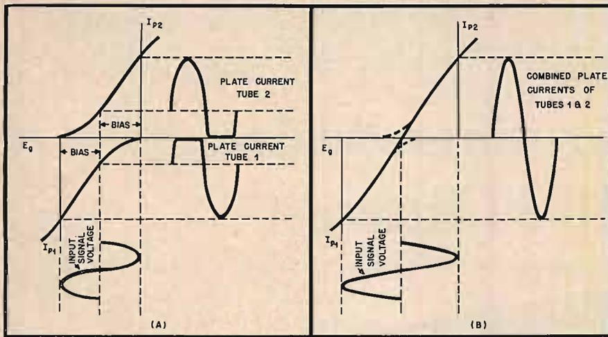
Fig. 12-22. (A) Transfer characteristics of two tubes in Class AB<sub>1</sub> push-pull. The two curves effectively combine into the single curve of (B).
