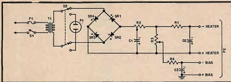
Fig. 2. Schematic of the d.c. power supply.
