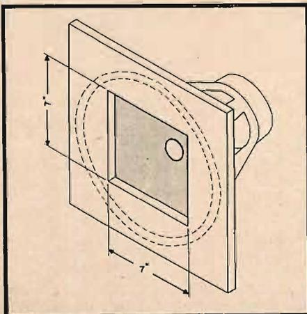
Fig. 8. Throat for low-frequency driver.
