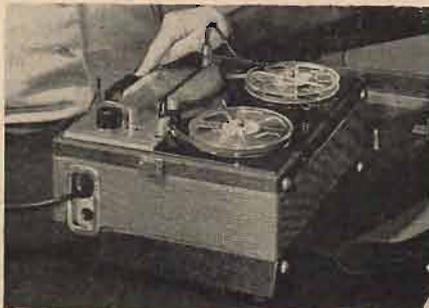
14 x 12 x 9 ins. Capable of using all sizes of tape spools up to 7-ins., the dual-speed machine can record or play back up to two hours, and can be rewound in approximately two-and-three-quarters minutes. Operating speeds are 3¾ and 7½ ips. The recorder is equipped with both input and output jacks to permit easy attachment to phonographs, radio tuners, and public address systems. Engineering Products Department, Radio Corporation of America, Camden, N. J.
