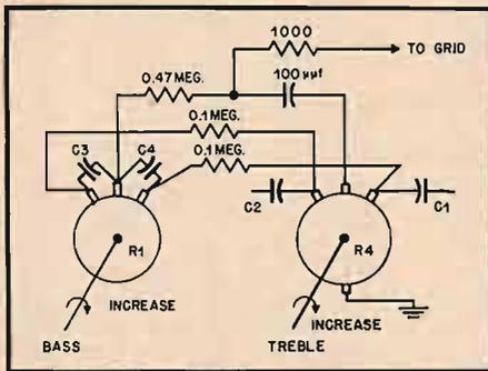
Fig. 5. Suggested wiring arrangement for the tone control. The two potentiometers R<sub>1</sub> and R<sub>4</sub> could easily be combined as a concentric control.
