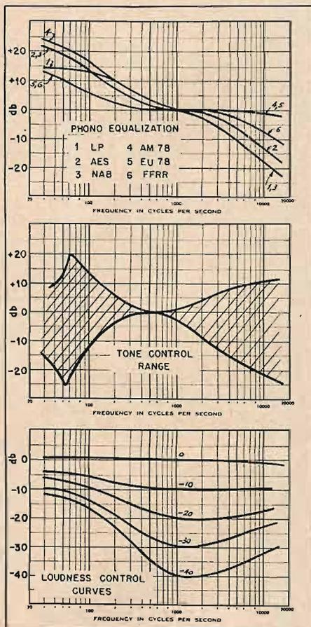
Fig. 3. Performance data for Bogen R701 tuner.
