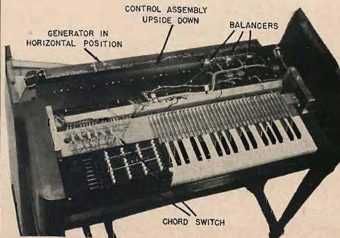
Fig. 10. Front view with the key section exposed.
