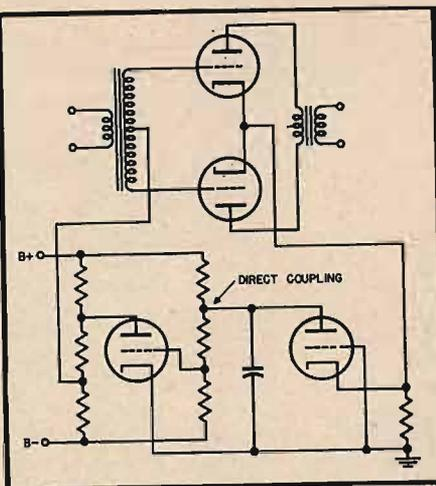
Fig. 12—24. Automatic bias control providing progressive transition from Class A<sub>1</sub> through Class AB<sub>2</sub> operation.
