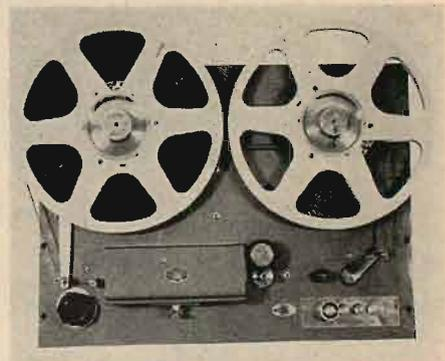
meter can be accommodated and recording speeds are 7 1/2 and 15 ips. Brakes and capstan pressure pulley are actuated by solenoids, making the RS-11 ideal for remote control. Presto Recording Corporation, Paramus, N. J.
