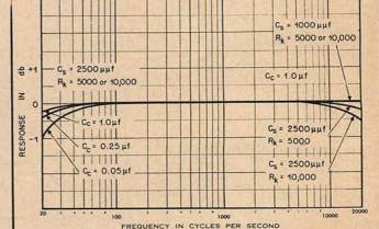
Fig. 4. Curve showing change in car-tridge response with change in a load isolated by a cathode follower.
