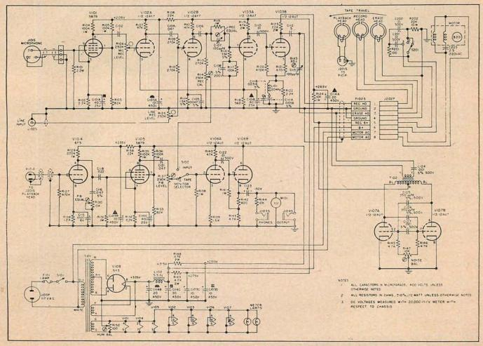
Fig. 7. Complete schematic of the Ampex 600 recorder.
