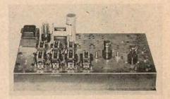
Fig. 8. A tone-changer chassis. The relays are actuated by the tabs, and act to provide different tone qualities as indicated by the stop tabs actuated.
