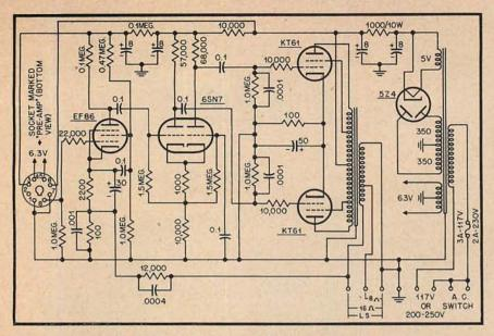
Fig. 4. Schematic of the Leak TL/10 power amplifier.
