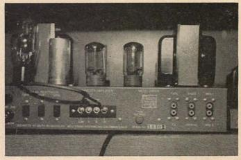
Fig. 1. In this "switchboard of home entertainment, six input sockets give your audio system extreme flexibility, accommodating Pickering pickup in Mag-1, GE and Audax in Mag-2, crystal in Xtal; in addition, there are radio, television, and tape recorder inputs.
