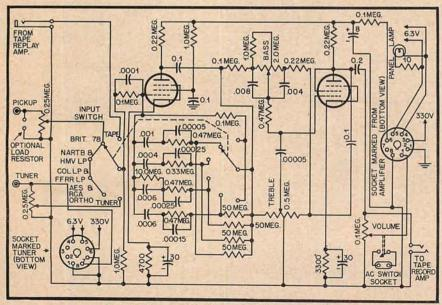
Fig. 3. Schematic of the preamplifier-control unit.
