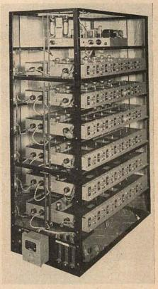
Fig. 5. External generator rack employed with some of the larger Allen models. Each of the six chassis shown carries seven octaves of two adjacent tones, or a total of 85 notes. (Eight octaves of the C tone are provided to include the top C of the scale.)
