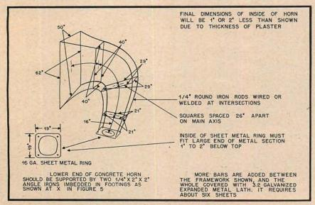
Fig. 6. Basic framework of 1/4-in. rods used as reinforcement for the horn. Framework is covered with metal lath before cementing.
