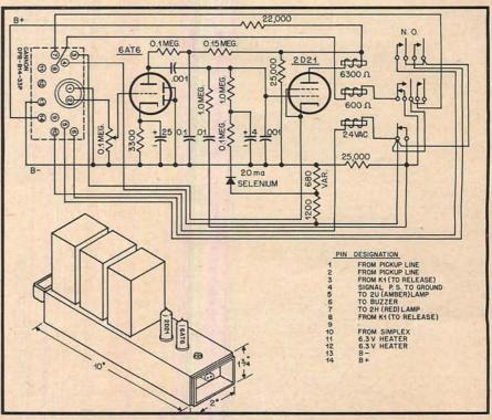
Fig. 2. Schematic and general appearance of one of the Channel Identification Amplifiers.
