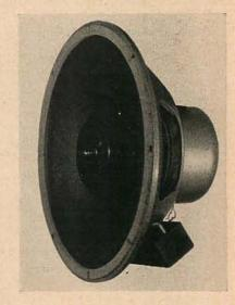
through a fully-enclosed magnet structure using 1½ lbs. of Alnico V, providing faithful response down to 40 cps. Coupled through a 5000-cps high-pass filter network are a Dural diaphragm and a 1-in. voice coil giving smooth response to 18,000 cps. Copper voice coils are used to approach the ideal ratio of conductor mass to that of the moving system. Power capacity is 20 watts. Impedance is 12 ohms. Stephens Manufacturing Corporation, 8538 Warner Blvd., Culver City, Calif.
