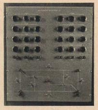
circuits, leaving them free for normal substitution use. The P100 will find wide application in the development of equalizers, attenuators, feedback networks, coupling circuits, voltage dividers, phase shifters, and time constant circuits. Full information will be supplied by the manufacturer.
