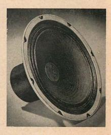
closed-back cabinet with internal volume of 1.7 cubic feet or larger, Constructional features include an aluminum voice-coil form to eliminate humidity and temperature variations, prevent warping and buckling, and to provide increased power-handling capacity. Flux density is 13,000 gauss and input impedance is eight ohms.
