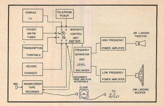
Fig. 3. The audio system that grew. This is the plan for a specific home installation, but any other combination of makes and types of equipment could be connected together in a similar manner to give great operating flexibility and a wide variety of audio services.
