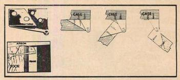
Fig. 5. Non-mortising type of semi-concealed hinge. Note the manner in which this hinge is installed. At the right the door is shown in closed, half-open, and fully-open positions.
