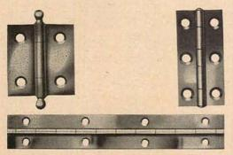
Fig. 3. (Upper). Two types of hinges. At left is a ball tip loose pin butt, and at right is a similar hinge less the ball tips. Fig. 4 (lower). Continuous or piano hinge which is available in lengths up to 72 in. and from 1 1/16 to 2 in. wide when opened out.
