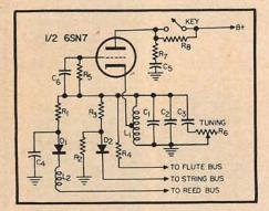
Fig. 3. Oscillator-filter circuit for one note.
