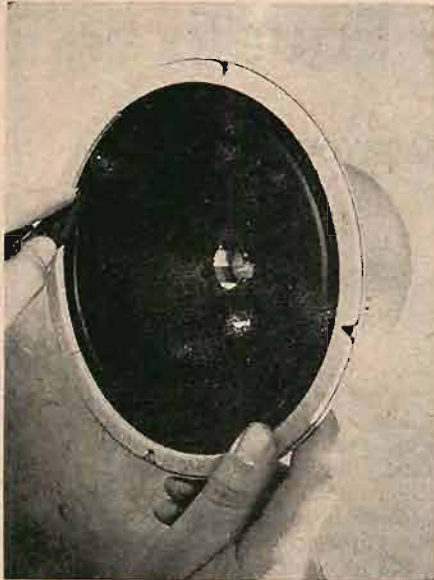
Fig. 4. Slitting the outer edge of the cone to remove it from mechanical engagement with the frame.
