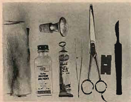
Fig. 1. Materials needed for treating speakers—chamois, solvent, cement, tweezers, scissors, razor blade, scalpel, and in some cases clothes-sprinkler head.
