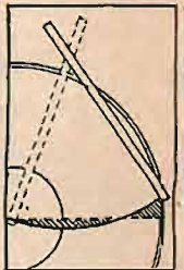
How Conventional Tone Arms Create Tracking Error (See Shaded Area).
