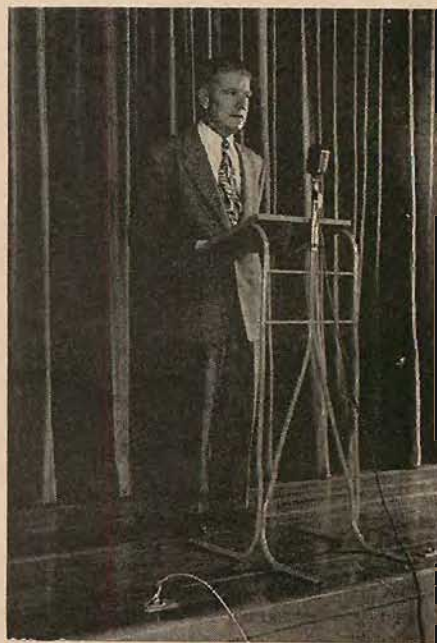
Fig. 3. "Keepaway" mike and manuscript stand which prevents speakers from hugging the mike.
