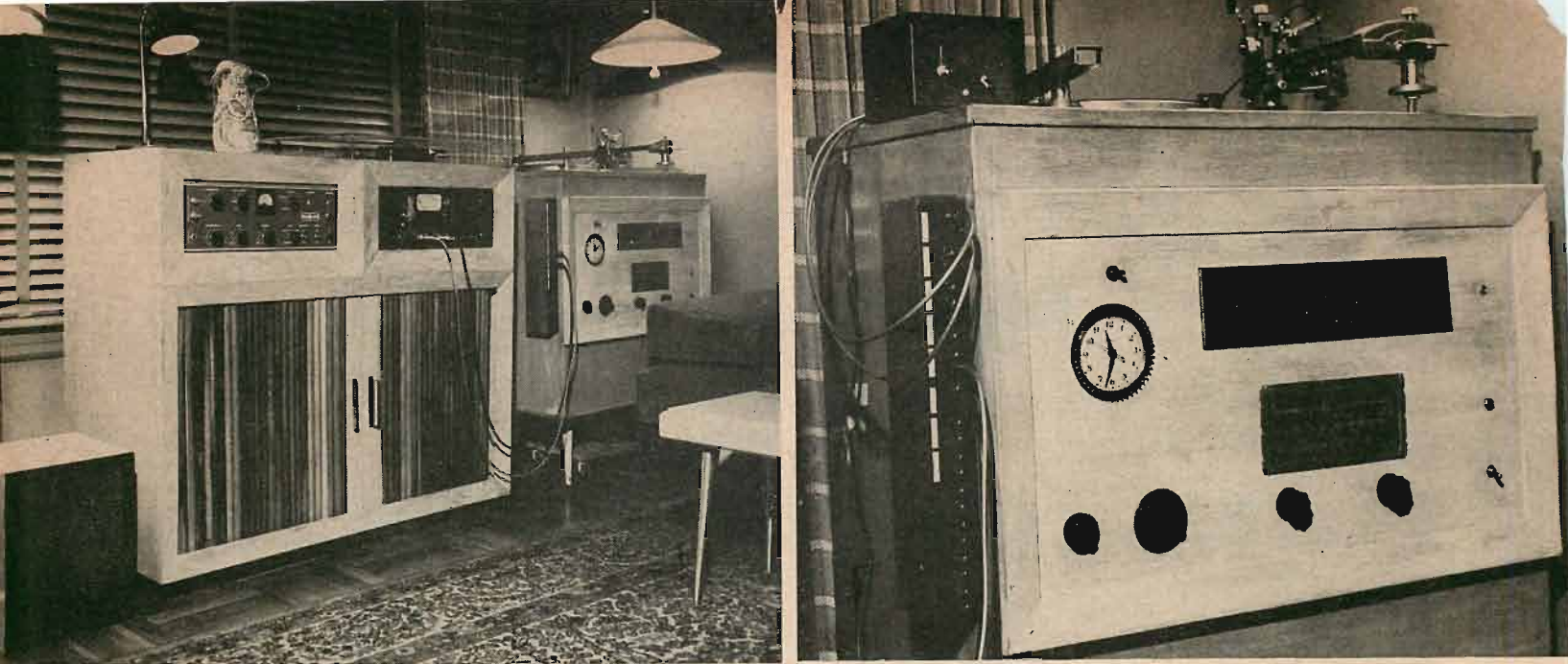
Fig. 1 (left). Setup of versatile hi-fi audio system along window-wall of 14 by 19 living room shows center cabinet housing recording amplifier and tape recorder; second cabinet houses record turntable and recording head, preamplifier, tuner, automatic clock, jack panel for patch system. Small cabinet lower left contains auxiliary speaker system, used also for monitoring recording amplifier in addition to headphones. Fig. 3 (right). Closeup of patch system strip showing insertion of hi-lo filter between pickup arm cartridge and preamplifier input. Clock is peg-controlled for presetting listening, recording or playback functions. Each peg represents 15-minute interval, providing precise programming and scheduling. Toggle switch over clock kills entire system.
