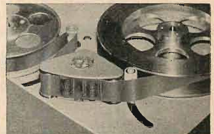
Data recording equipment uses two multi-channel Brush heads to record 25 data channels on a 1-inch tape.
