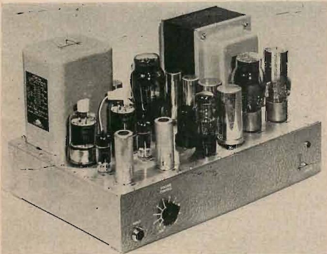
Fig. 3 (above) Schematic of the HF-40 amplifier, and Fig. 4 (left) its external appearance.
