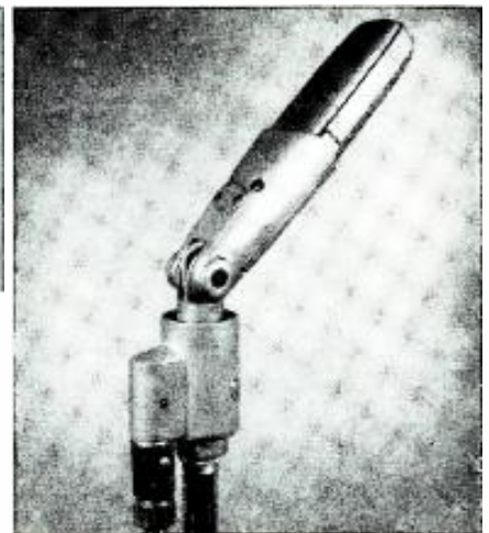
Above: The bi-directional pattern of the pickup plus the tilting feature will reduce unwanted noise and allow a PA system to be run about 6 db higher than usual when the "dead" sides of the mike are properly oriented in relation to the sound source. Right: showing the cable connection and impedance switch cover.
