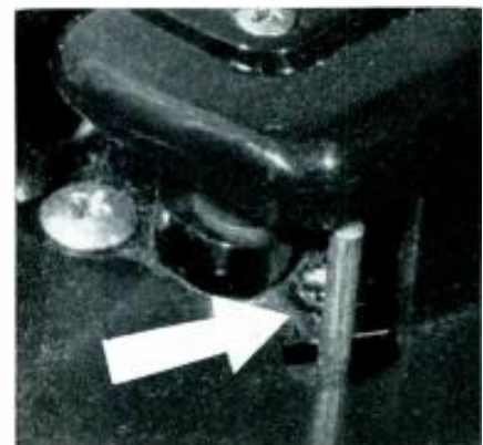
Above: the connection outlets are on the back of the recorder. Right: the pins which will shut off the recorder at the end of the tape if a loop has been formed around the hub of the reel.
