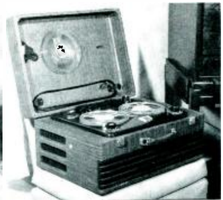
The line and microphone cords are wrapped on cleats in the lid and extra reels of tape are stored on the spring pins.
