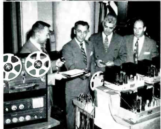
Upper left: the equipment used in the demonstration consisted of two recorders, ten 50 watt Fisher amplifiers and ten Jensen Imperial speakers. All the items were mounted in full view of the audience who were thus treated to an inside view of how recordings were made. Top right: the Western Electric 640 AA condenser microphone which made the orchestra pickup was suspended about 20 feet above the stage and slightly behind the podium. With it were rigged other mikes to provide a safety factor in case of failure. The 640 AA was calibrated by the Bureau of Standards. Center: the recorders and amplifiers were set up on the left side of the stage. This shot, made at rehearsal, shows the ten Jensen Imperial speakers lined up along the rear wall behind the musicians. Below: the principals in the production of "Soundorama." From left to right, Bert Berlant, president of Berlant Associates, Dr. Howard Mitchell, conductor of the National Symphony Orchestra, Harvey Fisher, president of the Fisher Radio Corporation, and Karl Kramer, manager of technical services of the Jensen Manufacturing Company.
