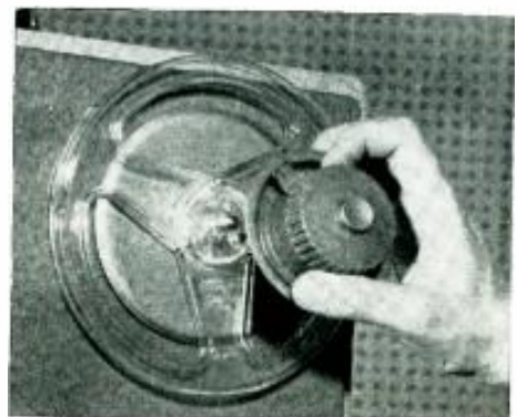
Reels are held in place with the "Reelok" which clamps on the shaft when the center button is pressed. Tab near edge releases it.
