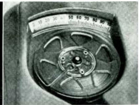
An accurate scale, together with the log pad enables anyone to quickly locate any spot on the reel without difficulty.
