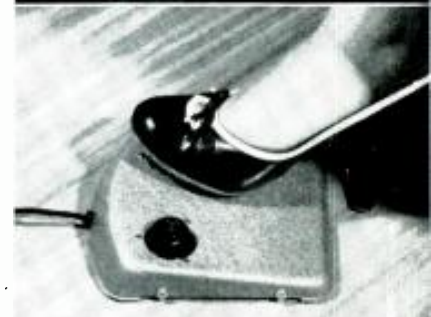
Top: the stethophone which the secretary wears for transcribing. Upper center: the telephone induction coil pickup, with its suction cup for attaching and the switching box to cut the machine to dictation or telephone pickup as desired. Lower center: the transcription control for typewriter. Bottom: the foot control for transcription.
