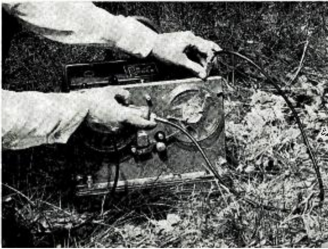
If you must run a long line, a microphone transformer should be used to match the impedance of the mike to the input impedance of the recorder. A low impedance mike and low impedance cable are best. If a high impedance mike is used, two transformers and a low impedance line are necessary.
