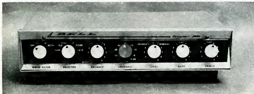
The Bell 3030 stereophonic amplifier is shown above. Rated at 15 watts on each channel, it can carry peaks of 60 watts. Variety of controls offers unlimited possibilities to sound diddlers.
