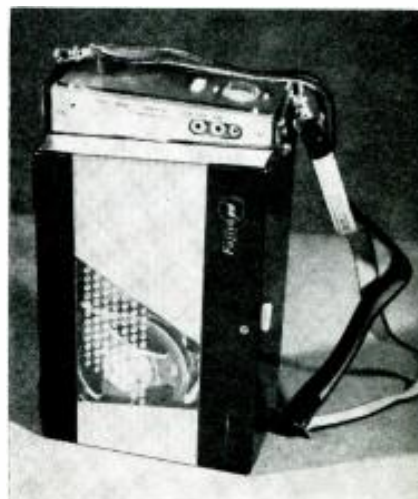
The recorder measures 9½" x 5½" x 3" and weighs four-and-a-half pounds. Controls are accessible when the case is closed.
