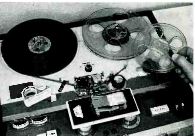
For the present, once we have our full-hour recording we will have to edit it down to "standard" 48-minute length so it'll fit on a 7" reel. Do this either by direct editing, saving the extra tape on a separate, smaller reel. Or (much better) by re-recording the hour tape, slimming it down to 7"-reel size electronically.
