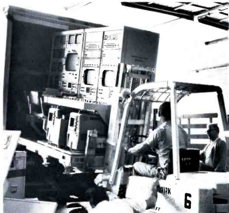
Fig. 2. The innards of the module fit nicely into the body of a standard rental truck. Note that it still rides on its skids. Note also the camera bodies stored below the desk of the console.
