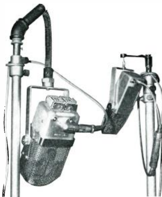
Figure 1. (Left) the Cambridge C-3 microphone and (right) the new C-4 model. These are ribbon designs with built-in solid-state amplification and emitter-follower outputs. The battery power supply for the C-3 is seen atop the microphone.
