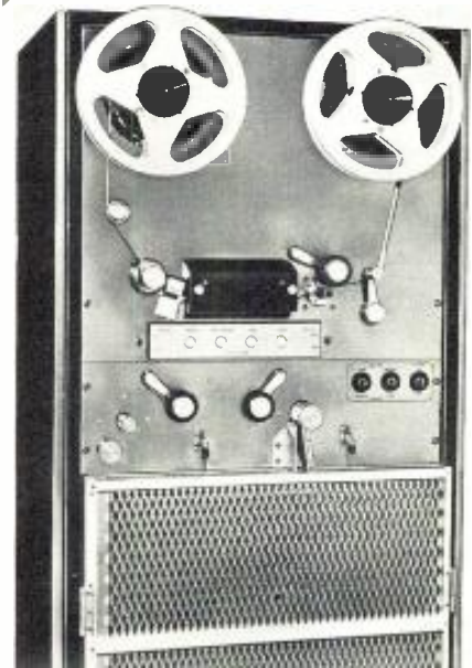
The Electro Sound master's bin permits the tape to be seen.
