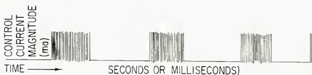
Figure 4. The wave-form of pulse bursts, useful for testing audio equipment and other experimental applications including electronic music.
