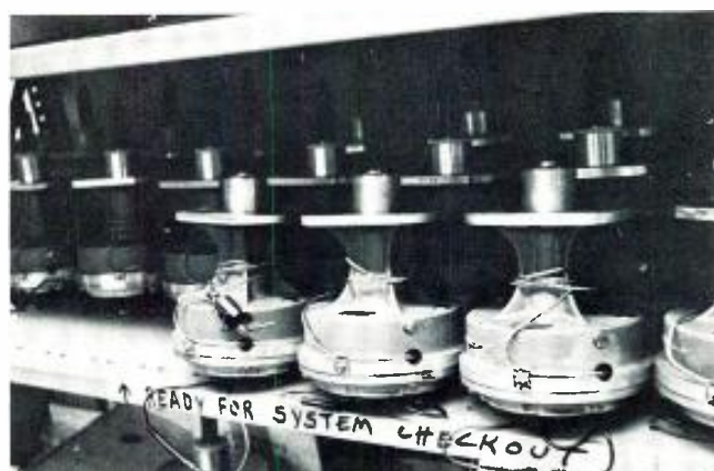
Special d.c. capstan motors used in the ABR stand ready for inspection.
