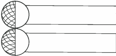
Figure 3. Two matched omnis can be used to assemble a quality differential mic.
