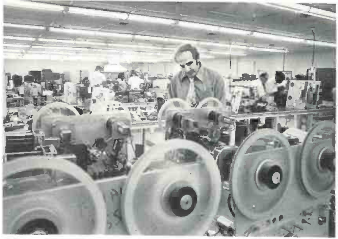
In other parts of the plant Scully 270 models are being assembled. This is a test station.
