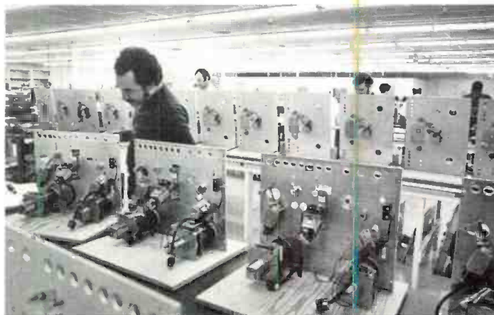
A technician checks partly finished 280 transports as they progress along the line.
