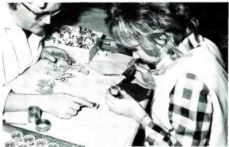
Wire leads are attached to the pre-assembled microphone element.
