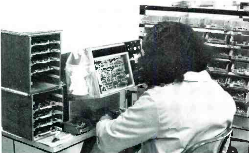
An ingenious light board is used for component location during assembly of circuit boards—in this case, for the Cat. 22 noise reduction boards. As each different type of component (e.g. 1k resistors) is required, the jig lights up to show the positions for that component at every location. In this way, the over 500 components on this board tend to get put in the correct place the first time around.
