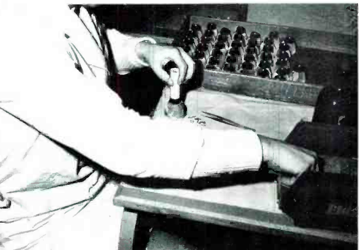
An acoustic tube is added during the assembly of this microphone.
