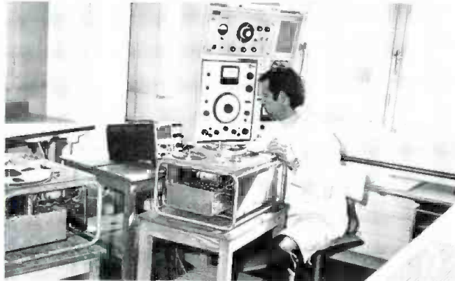
Studer B-62 units are still a big part of production. Here a completed one undergoes final adjustment.
