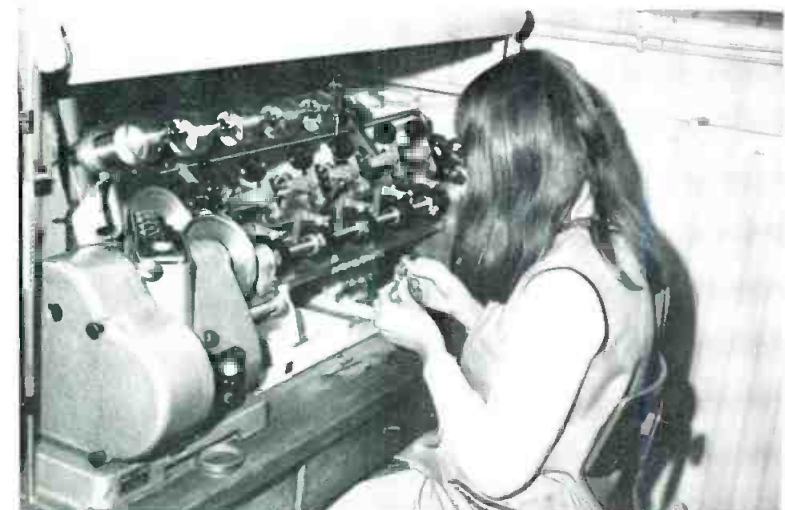
This highly sophisticated coil winder creates mic coils rapidly and with high precision.
