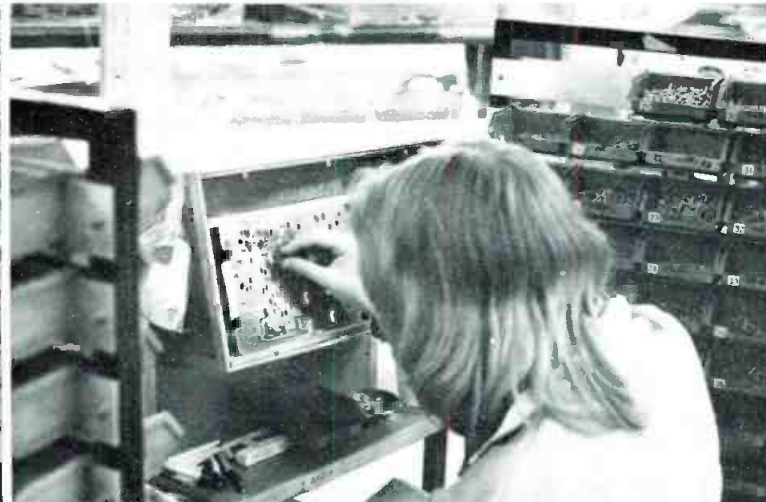
An ingenious light board is used for component location during assembly of circuit boards—in this case, for the Cat. 22 noise reduction boards. As each different type of component (e.g. 1k resistors) is required, the jig lights up to show the positions for that component at every location. In this way, the over 500 components on this board tend to get put in the correct place the first time around.
