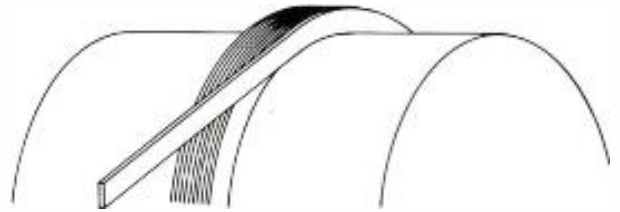
Figure 2. Method of winding loud-speaker voice coil with flat, rectangular wire, achieves better space utilization, and provides greater variety of impedance choice.
