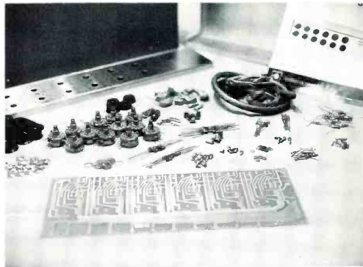
This is how it looks when it comes out of the box for a parts check. Most of the components go on the circuit board.
