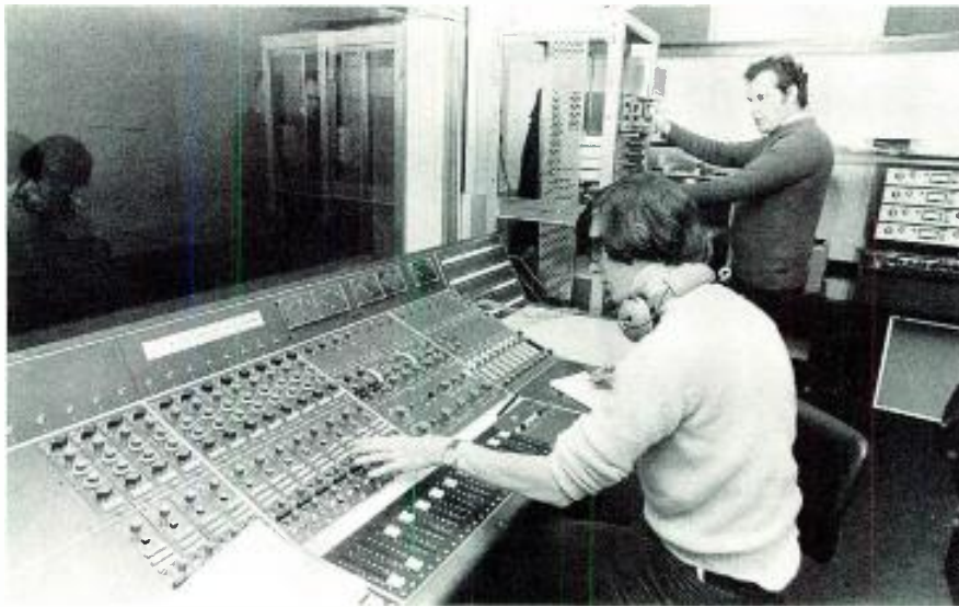
Figure 1. A view of the control room at Surrey University with its Neve board, four-track Scully, Dolby A units, and Spendor speakers.
