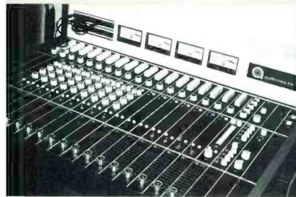
The grandson of 36 grand from Audiotronics is a compact 18 in, 4 out console design. Circle 59 on Reader Service Card.
