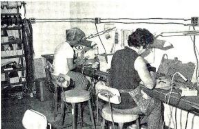
In this group, various stages of component assembly are seen. The skilled women workers handle a large part of the individual assembly, rather than strictly working on a pass-along basis—though this technique is also used.
