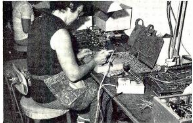
In this group, various stages of component assembly are seen. The skilled women workers handle a large part of the individual assembly, rather than strictly working on a pass-along basis—though this technique is also used.
