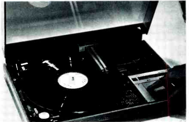
This is a completely automated B & O turntable with a straight-line tracking arm.
