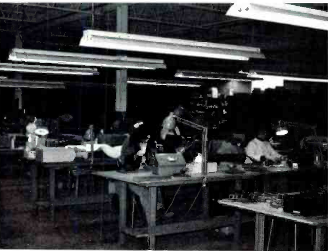
A modified assembly line system is used for modules. Each individual station is responsible for the major assembly.
