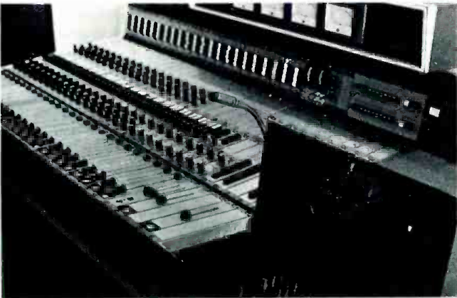
The Schlumberger console with its interesting patch bay.
