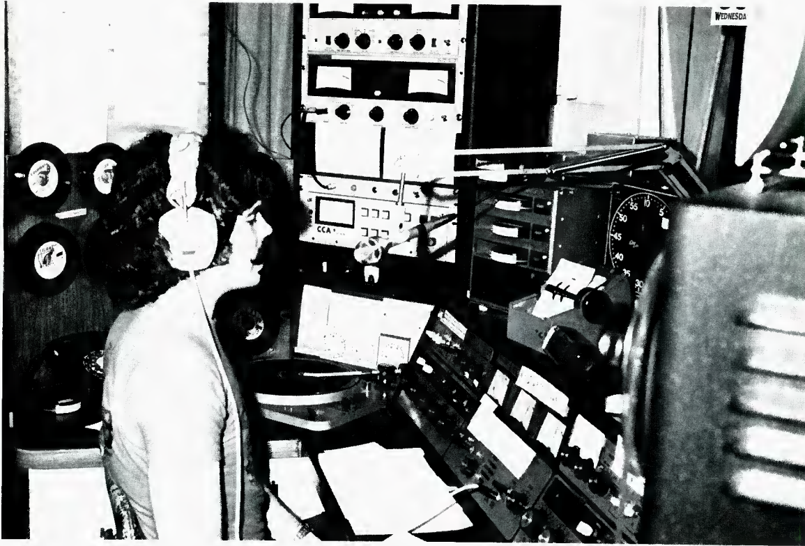
Disc jockey Jim Collins, who is in charge of the 2-6 p.m. program, is at work in the main control room. In front of him are six stereo cartridge decks used exclusively for all on-air material.
