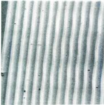
A general view at approximately 45 degrees to the surface. The vertical and lateral shifts of the groove and the deviations of the f.m. signal superimposed on them can easily be seen. Although this record was new and apparently clean, dirt particles are very noticeable. (X100)
