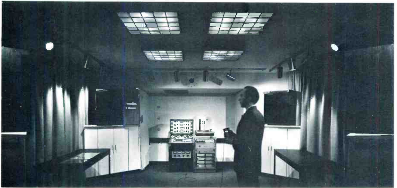
The listening room at the Center. A remote switching box permits comparisons between SQ encoded and discrete tape sources playing from the turntable or half-inch Scully tape machine.
