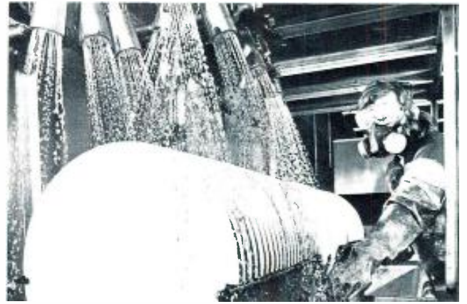
Figure 2. After being lapped perfectly smooth, the aluminum blank is etched and cleaned to provide a hospitable surface for lacquer coating. This is the final cleaning process.
