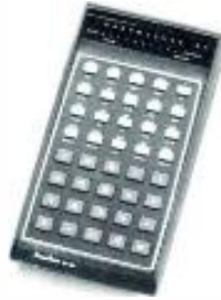
The Kingspoint SC-60. All basic scientific functions are directly available with the forty keys used. The shift key must be used to utilize supplementary convenience functions.
