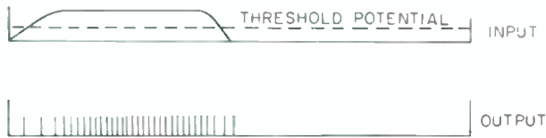
Figure 3. A time record of sensory excitation. Stimulus causes a rise of receptor "generator potential" until it exceeds threshold potential, whereupon it creates pulses of "action potential" in a nerve.
