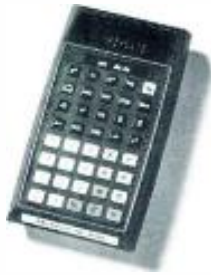
The Melcor 635. Note the forty-key layout utilizing all single-purpose keys. This unit can display exponents even though they are not shown on the readout.
