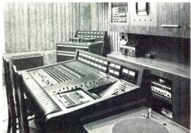
The control room, with the 19-in, 16-out console, MCI 16-track, dbx, and Dolby units at hand.
