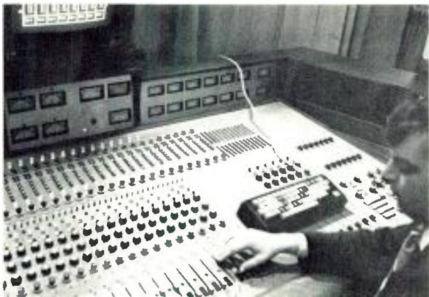
Figure 8. The Quad-Eight console, as equipped with the Compumix III automation system.
