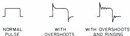
Figure 2. A transient appears as an overshoot, sometimes with ringing.
