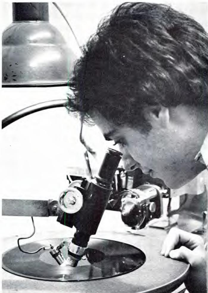
A student inspects freshly recorded grooves in the school's disc recording lab.
