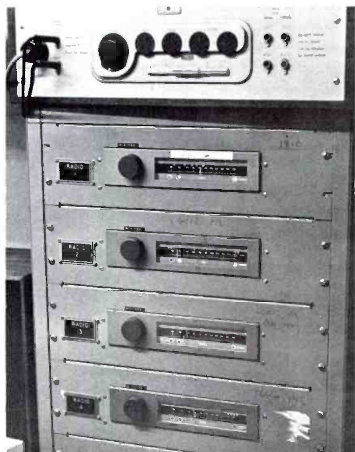
A rack full of quad f.m. tuners for BBC air checks, tied into the automatic time clocks for unattended off-air recording
