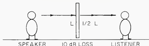
Figure 2. A vertical barrier (screen) reduces by at least one-half loudness the transmission of sound.
