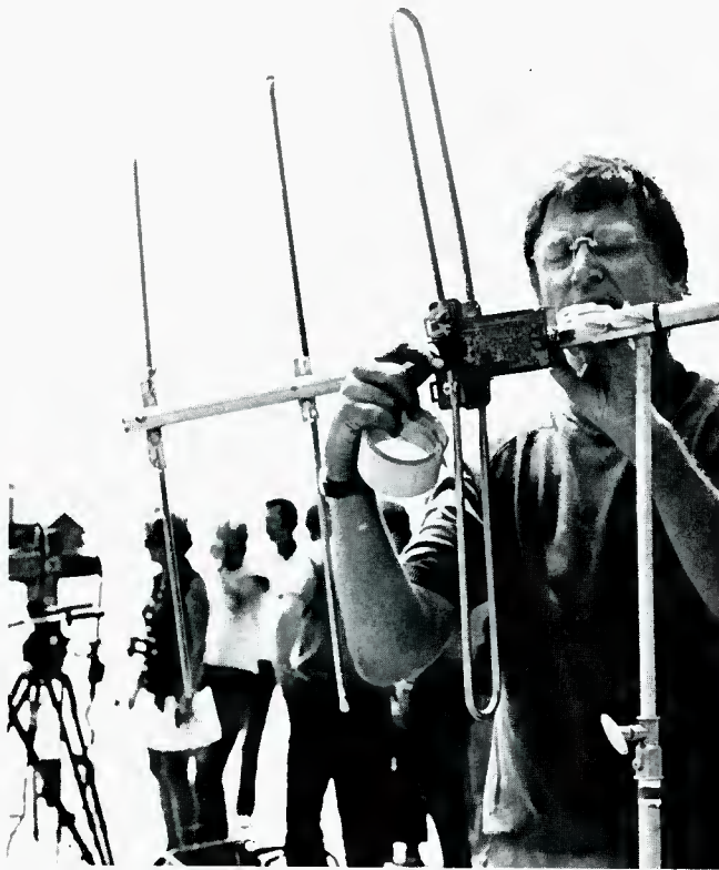
A wireless microphone being prepared to be used in a field remote where the performer will move across open ground.
