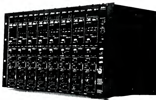
The Shared Access Memory System shown with 8 pitch/delay modules installed in the mainframe.
