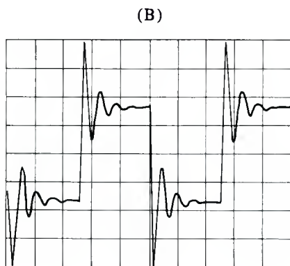
Figure 5. (A) A set of reciprocal (non-constant-Q) frequency response curves. The curve shape tends to become "peaky," and the bandwidth increasingly narrow as the boost is increased. Compare these curves with the constant-Q family seen in Figure 3(A). (B) The reciprocal equalizer's square-wave output for a 10 dB boost. Note the large amount of ringing, and
