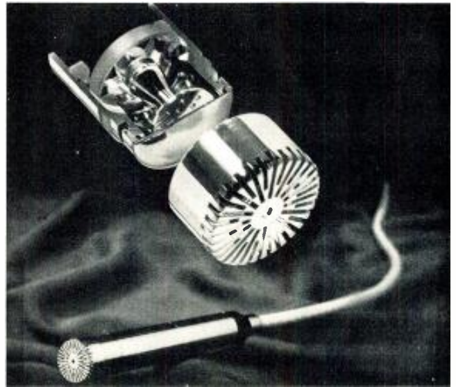
Figure 3. A Bruel & Kjaer 1-inch, free-field microphone, Type 4145.
