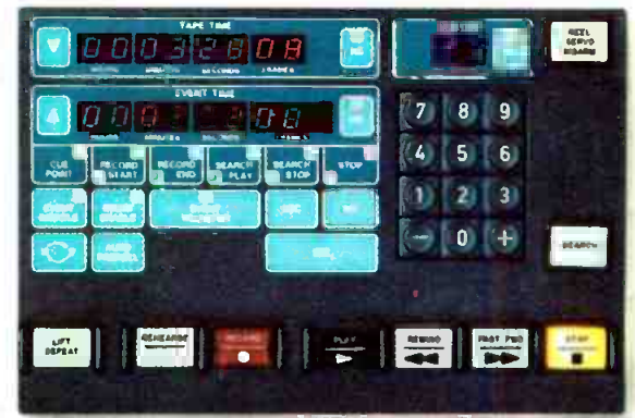
ATR-124's Multi-Point Search-To-Cue (MPSTC). Provides 100 cue locations.
