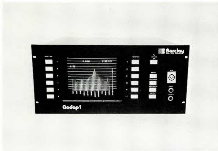
Figure 1. Badap 1 Audio Micro Computer.
