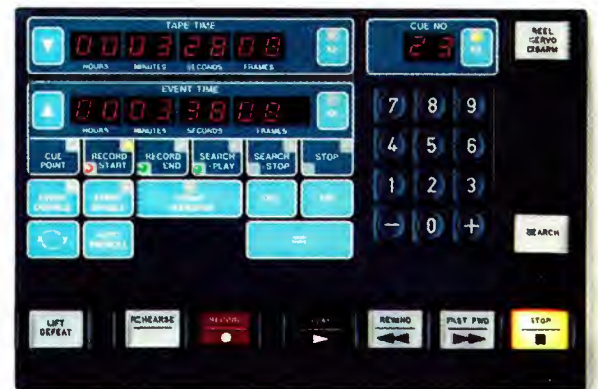
ATR-124's Multi-Point Search-To-Cue (MPSTC). Provides 100 cue locations.
