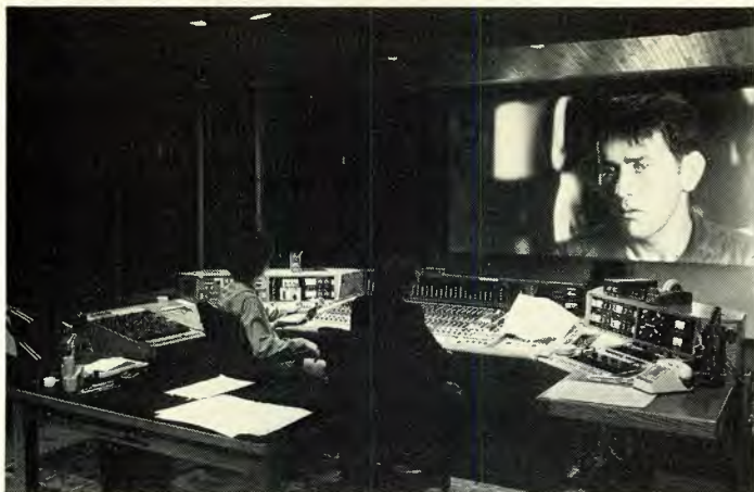
The sound track for Apocalypse Now was mixed on an automated MCI 24-track console. The great majority of cinema-sound consoles now in use were created for and often by the film industry, however. Photo courtesy American Zoetrope.
